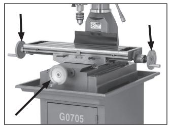
Figure 20. Table handwheel handles.
